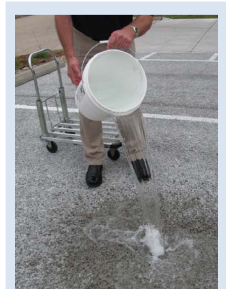
Porous pavement allows stormwater to flow through the pavement rather than runoff in large quantities.
